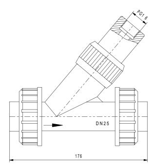
The bevel seat flow-through housing AD 82 is used for installation in piping and pre-eminently for insertion of a process dissolved oxygen probe. The special construction features optimal flow conditions for the sensor and a self-cleaning action for the membrane of the oxygen sensor.
