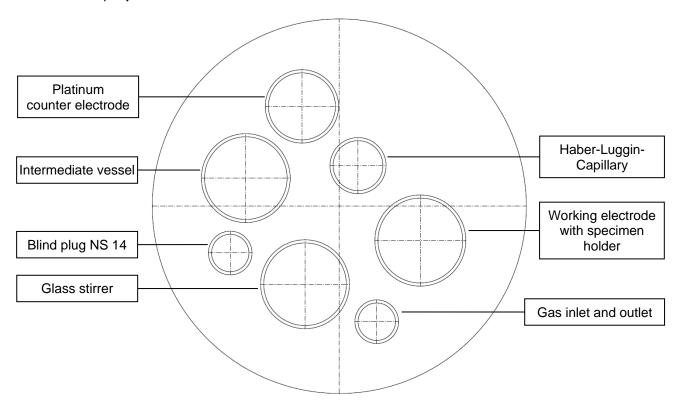
The outside diameter and the height of the glass container is 100 mm. The dimensions of the cell top: diameter 120 mm, height 35 mm. The specimen holder consists of two parts: polypropylene stopper with eccentric threaded bore M12x1 mm and a polypropylene specimen shaft with outside thread M12x1 mm for fixing inside. In the upper part of the specimen holder there is a jack for current entry and on the opposite side there is an outside thread M8 for fixing the sample.
